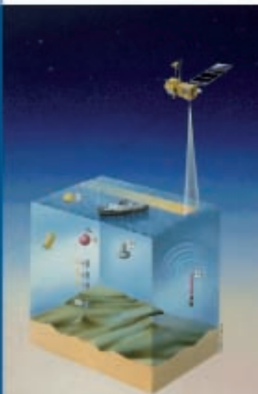
Ocean observation infrastructure: Surface vessels, moorings, drifters, satellites, ROVs, AUVs and sea-floor observatories
